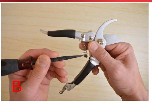
If the spring becomes dislodged using a small screwdriver it can easily be put back into place. Ensure the small end of gromet is exposed from the spring (Picture A). Then guide it into the handle (Picture B).
