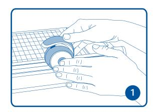
To remove the blade, push the button in the center of the blade cartridge
