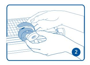
Grasp the edges of the cartridge and pull straight out
